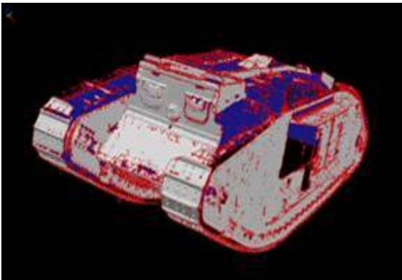
Figure 18. Locations of Missing Surface Data (in Red)
