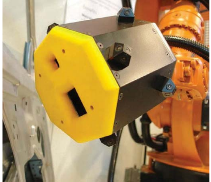
A Robotic MMDx scanner mounted to a robot replaces the hand-held version of the sensor.
